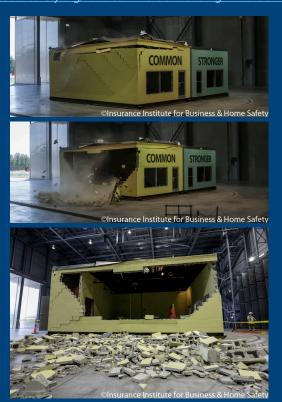
At a 105 mph wind gust, the equivalent to 85 mph oneminute sustained winds, the wall separated from the "common practice" building and the masonry side wall collapsed during the first full-scale high-wind test of commercial structures at the IBHS Research Center. two sets of IBHS FORTIFIED standards developed specifically for commercial construction and retrofit/repair:
